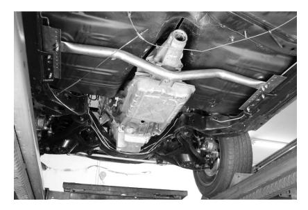
Install the crossmember frame brackets in the original factory bolt holes then mount the Crossmember. (64-67 convertible chassis shown here)
