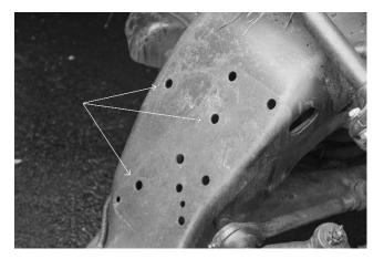
The frame brackets and engine mounts are marked for orientation. The frame bracket studs will be inserted into the top two of these holes in your frame.
