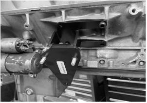
Start the 3/8"-16 nylon lock nuts and flat washers on the two studs that are attached to the frame brackets and through the frame but leave them loose at this time. After the assembly is in place slide the mounts into position.
