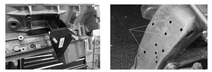
The frame brackets and engine mounts are marked for orientation. The frame bracket studs will be inserted into the top two of these holes in your frame.
