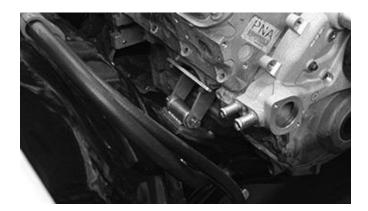
After the Crossmember is installed the frame and engine mount bolts and nuts can be tightened.
