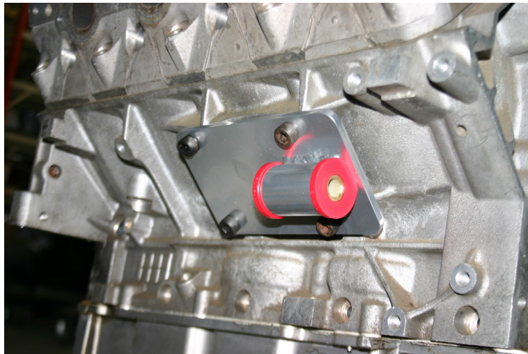
(Detailed view of passenger's side motor mount on engine)
