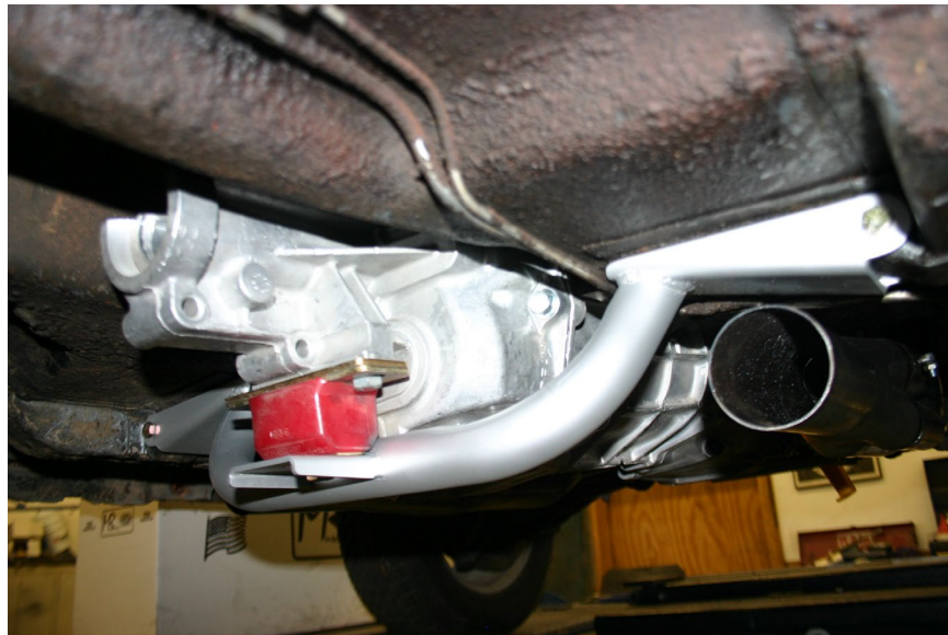
T-56 Crossmember (requires cutting open the transmission tunnel for transmission to fit)
