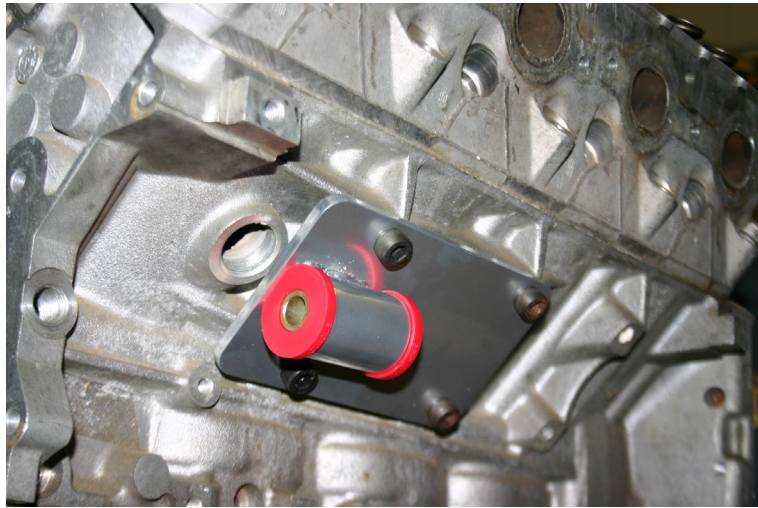
(Detailed view of driver's side motor mount on engine)
